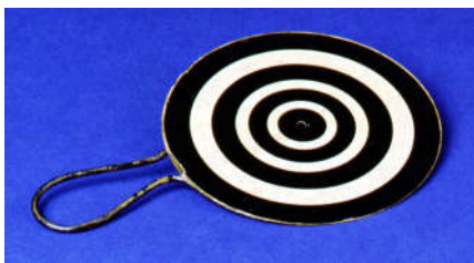
Fig. 1 Keratometer from 19th century for examining the anterior surface of the cornea [1]. It consists of a disk with concentric rings and hole in the center to view the reflection of the disk at the cornea surface.
