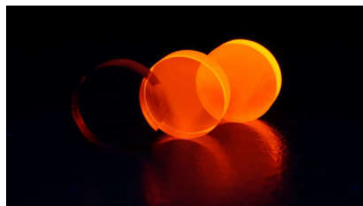
Fig. 1 From left to right: undoped, 0.46 at.%, and 2.29 at.% Eu^{3+} -doped borate glass discs under UV excitation.
