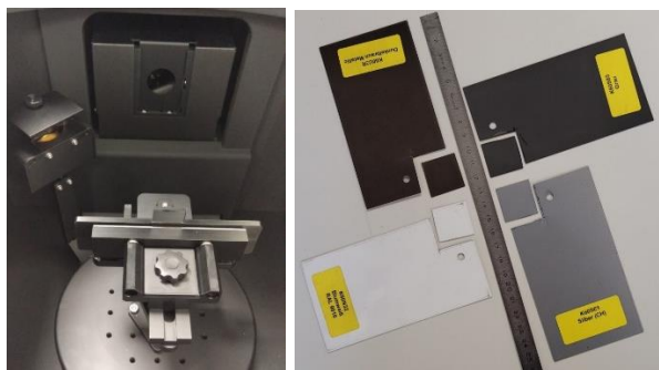
Fig. 5 Reflectometer in Wrexham Glyndwr University and samples with powder coating in different colours.
