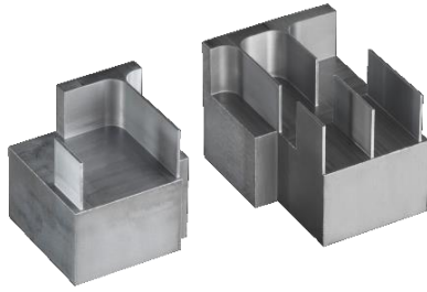
Fig. 3 : The abs-d x-ray interferometer after machining. The relative motion of the two parts is tracked by an interferometer using mirrors polished into the material on the other side.
